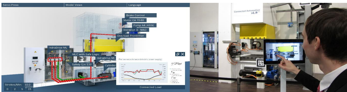
Figure 3. (a) 3D visualization of condition monitoring and simulation values, energy and data flows, product and process information of the press [10]. (b) Augmented Reality press connected to the real NC control [10].
