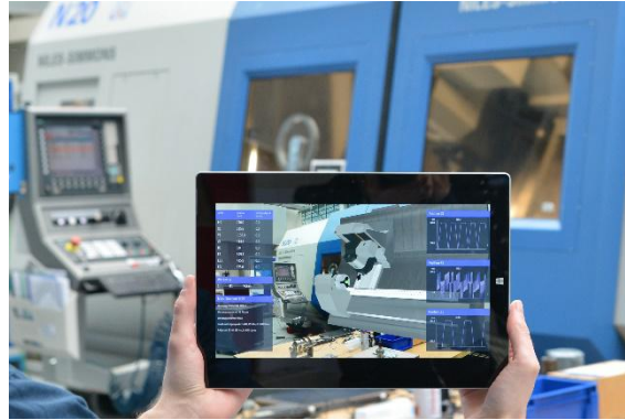
Figure 9. AR application for condition monitoring of machine tools with a synchronous virtual 3D model [10].
